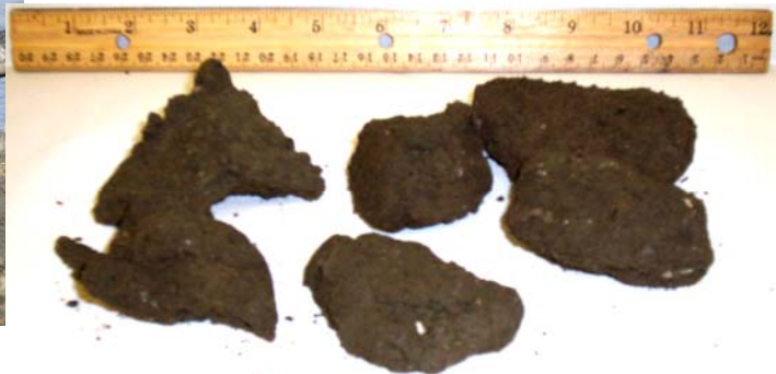
Organic sediment dewatered by vacuum bagging.
